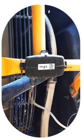
As a result, Tingz successfully implemented a system that could distinguish and categorize various activities of construction machines. This included differentiating between working, idling, loading, and the number of trips conducted by each machine.
